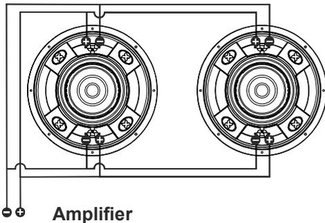
Parallel-Parallel 2x Dual 4 ohm subs = 1 ohm
